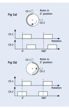
The second channel can be used to determine direction of rotation by comparing the phase of its input pulse with that of the first channel.
