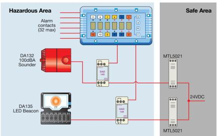
The LN1000 intrinsically safe alarm annunciator functions in the same manner and with the same operational logic as conventional flashing-light alarm panels.
