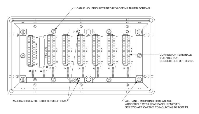
Rear view of the 12 way annunciator showing the terminals (Figure 9.1)
