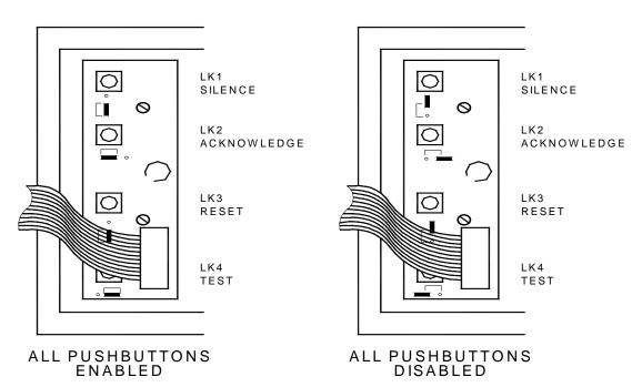
Jumper links on Pushbutton Card (Figure 14.2)
