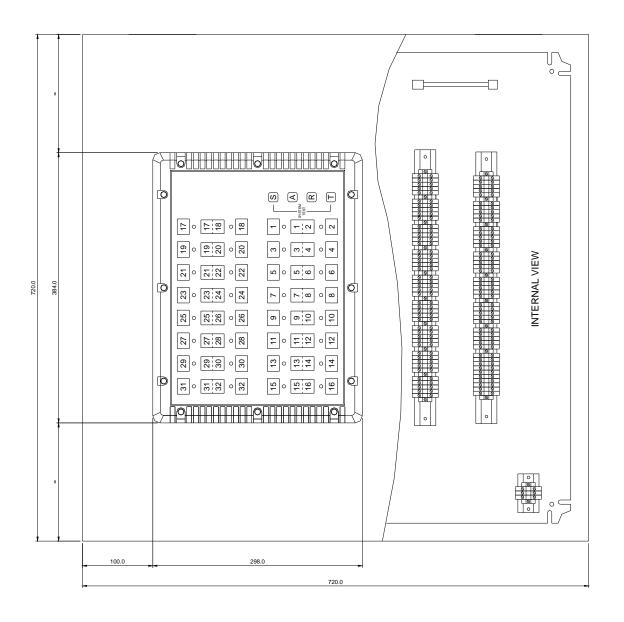
32 Way wall mounting Annunciator overall layout and dimensions (Figure 6.4)
