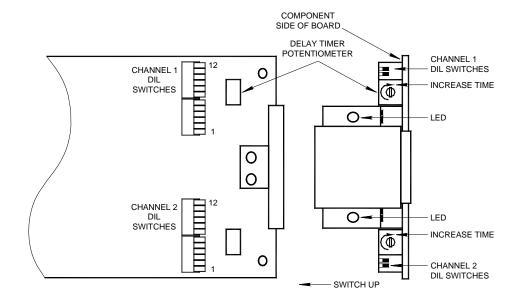
Alarm Card DIL switch and potentiometer location (Figure 14.3)
