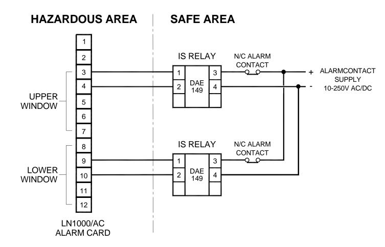
Alarm ways with normally closed contacts mounted in the safe area (Figure 12.3)
