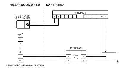
Connections to sounder using safe area mounted IS relay (Figure 13.1)
