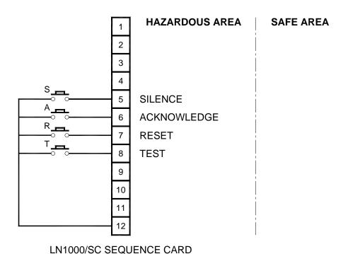
Remote pushbutton connections (Figure 12.5)
