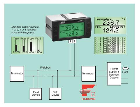
The BA688CF-F Fieldbus Display is a general purpose instrument that can display up to eight fieldbus process variables. Eleven selectable standard screen formats contain one, two, three, four or eight variables, with units of measurement, tag descriptions and bargraphs on some screens.
