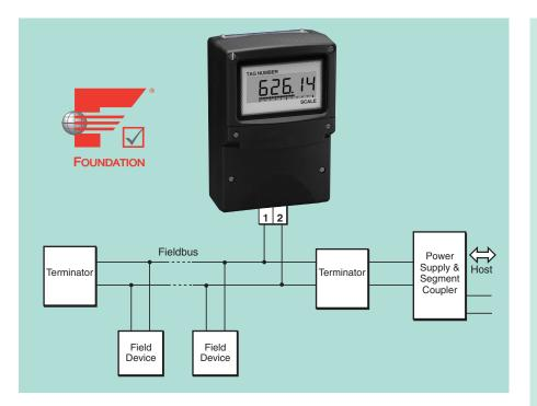
The BA614DF-F Fieldbus Indicator is a new cost-effective field mounting instrument that displays a single fieldbus variable in a process area. Housed in a robust IP66 GRP enclosure, the instrument has a large, high contrast five digit display, plus a horizontal bargraph. The BA614DF-F indicator uses the same technology and compliments the well established BEKA eight variable fieldbus displays that are now in worldwide use.
