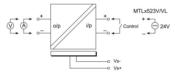
Figure 2 Basic test arrangement - separately powered
