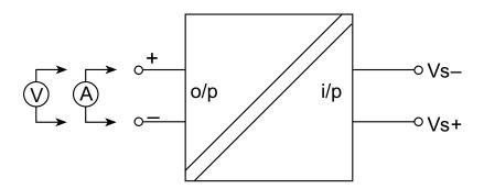
Figure 1 Basic test arrangement - loop powered
