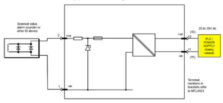
The MTLx52x modules are designed to power a field device such as a solenoid valve in the hazardous area and are driven from a safe-area source. The yellow (hatched) area shows the safety relevant system connection when using the loop-powered configuration. For simplicity the term 'PLC' has been used to denote the safety system performing the driving function of the process loop.
