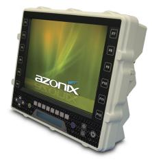
Azonix has developed a new glass base projected capacitive touchscreen with an enhanced optical interface that can be operated with gloves. The glass base front will not discolour with time nor is it as susceptible to scratches as are other non-glass based touchscreens.
