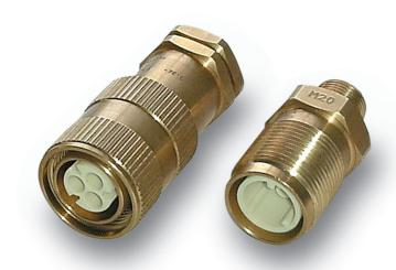
MTL951 Ex d e Hazardous area plug and socket connectors enable the operator to remove equipment from a power or signal line in a hazardous area, without having to isolate the supply. It also allows fieldbus equipment to be removed from the bus without having to disrupt communication with other equipment attached to that bus.
