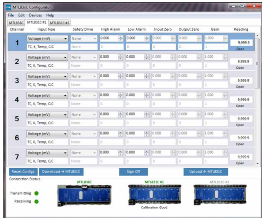
Figure 4- MTL838C with one MTL831C connected configured TC, K, Temp, CJC
