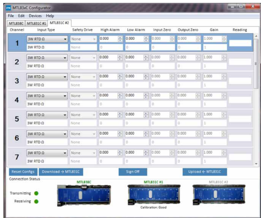
Figure 7 - MTL831C#2 tab while connected to an MTL838C and MTL831C #1
