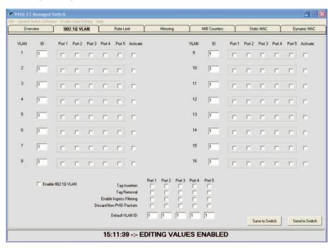
As can be seen on the above screen the 16 VLANs can be configured with an ID, port members and whether currently active.
