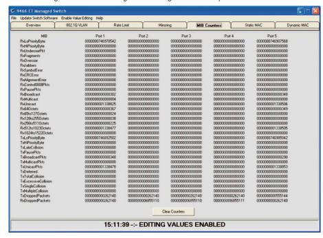
Use the button at the bottom of the display to zero the MIB counters and remove earlier stats.
