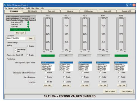
To the right of the status is the port usage. This provides an easy to view insight into the amount of throughput on the switch and whether the Ethernet Architecture needs any maintenance.
