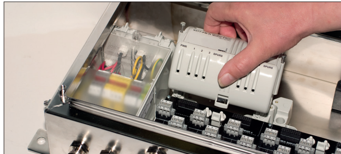
Figure 5.1 - Fieldbus Barrier module – fitting & removal
