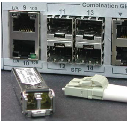
This image shows a typical SFP/LC transceiver and dual-LC cable.
