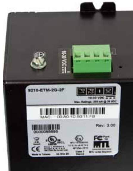
Figure 4.1 - Power connector and grounding screw
