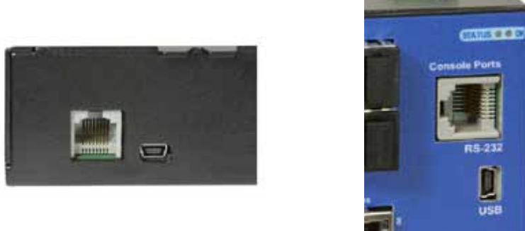
Figure 5.2 - The RS232 (RJ45) and mini USB ports
