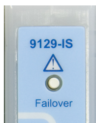
Figure 5.1 SAM failover switch
