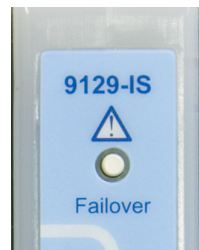
Figure 5.1 SAM failover switch
