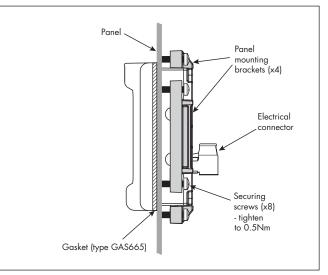
Figure 18 Panel-mounting MTL665 display
