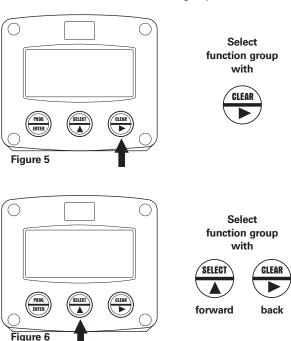
Each function has a unique number, which is displayed below the word "SETUP" at the bottom of the display. The number is a combination of two figures. The first figure indicates the functiongroup and the second figure the sub-function. Additionally, each function is expressed with a keyword.
