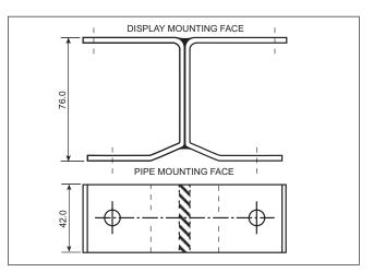
Figure 15 PIP66 kit - dimensions guide
