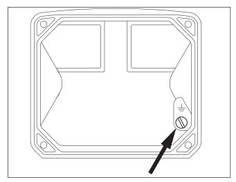
Figure 11 - Grounding aluminium enclosure.
