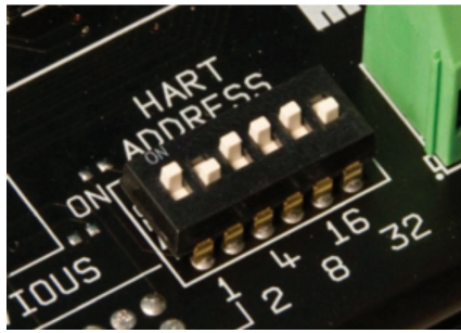
Figure 5.2 – Typical HART address switches set to address '29'
