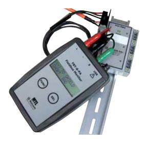
button. The first device shown will be the Master. By default, measurements greater than 150mV are OK. If a device leaves the segment, a "-" is displayed; if a device is added it shows "+".
