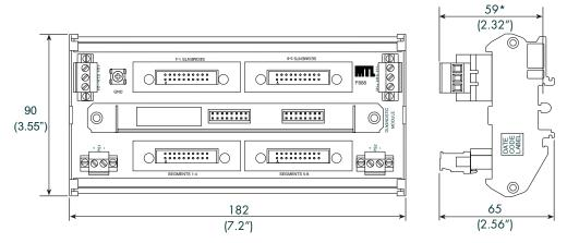
\* 175 (6.9") from DIN rail with F809F fitted
