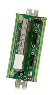
The F888 carrier is a compact, low cost, DIN-rail mounting solution for the F809F diagnostic module. It provides integrated fieldbus physical layer diagnostics with the Yokogawa ALF111 fieldbus communication module and any fieldbus power supplies.
