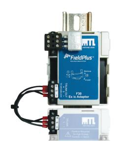
The F30 Ex ic Adaptor is an accessory to F300 Series Megablock wiring hubs, and provides intrinsically safe Ex ic spur connections for fieldbus networks in Zone 2 hazardous areas. One F30 is used with each Megablock, to limit the voltage at the spurs to Ex ic levels. When connected to suitably certified fieldbus instruments, the spurs may be live-worked in accordance with normal intrinsic safety procedures. The F30 is completely transparent to all fieldbus communications.
