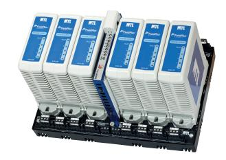
The 919x-FP module provides galvanic isolation between the 24V DC input power and the fieldbus segments, as required by the IEC61158-2 fieldbus standard and the Fieldbus Foundation™ FF-831 validation test for power supplies. There is also galvanic isolation between the fieldbus segments, thereby preventing multiple segment failures due to ground faults on more than one segment.
