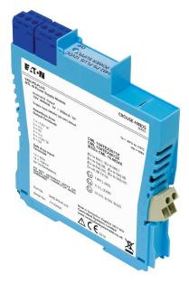
The 9492-PS-PLUS module has LED power indication for both input and output along with internal current limiting and electronic auto-reset circuit breaker action to protect the module in the event of its output being short circuited or overloaded. This also minimises the power dissipation during the fault to a negligible level, thus improving reliability.
