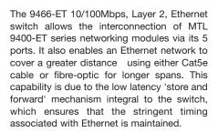
With the 9466-ET switch each connection is effectively a 'point-topoint' network segment unlike the older generation hubs that were simple 'dumb' repeaters. The old hubs needed to impose a limit on overall network length to ensure proper collision detection; this limit is overcome by the 9466-ET. Broadcast "storm" protection is also provided to eliminate network overload due to excessive 'broadcast' & 'multicast' packets.
