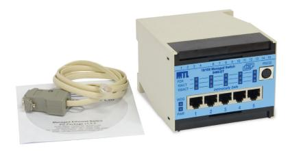
The 9466-ET switch can also distribute power to compatible devices connected to each of its five ports via the RJ45 Cat5e cables (PoEx). This method eliminates the separate power supply cable to the device simplifying installation and maintenance.
