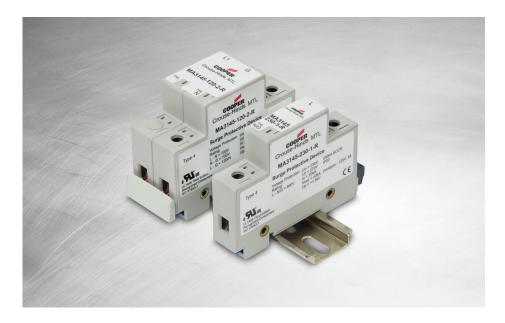
**The Class II surge current arrester** is designed to work as both a standalone device and in cascade coordination with MTL's Class I lightning arrester. A single width module withstands surge currents up to 40,000A with an 8/20µs waveform. Class II arresters are available in single width modules for maximum user flexibility, double width modules for all-mode protection on single phase systems and quad width modules for all-mode protection on three phase systems.
