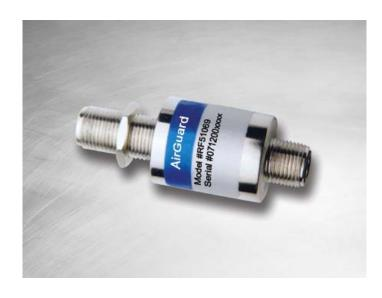
The FGT Series of surge protection devices prevents surges and transient overvoltages conducted through coax cables used for wireless Local Multipoint Distribution System (LMDS), Wireless Local Loop (WLL), and Multichannel Multipoint Distribution Service (MMDS). These versatile products can be used in any "F" connector application from DC - 2.5GHz frequencies to 75 ohm impedance.
