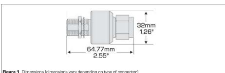
Figure 1 Dimensions (dimensions vary depending on type of connector)
