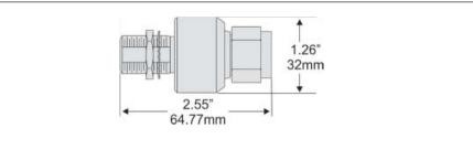
Figure 1 Dimensions (dimensions vary depending on type of connector)
