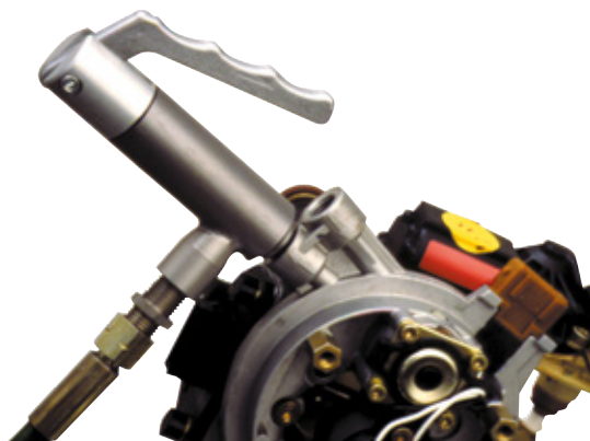
TW17H | Testing of injection pumps
