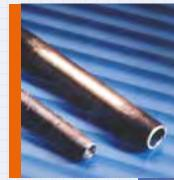
Tungum Tubing remains unscathed despite more than 10 years marine exposure on a semi-submersible support vessel. The Stainless Steel section, from a southern North Sea platform, shows both crevice corrosion and chloride pitting after barely 5 years in the same environment.
