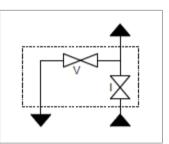
• Type E/F Outlet 1/2" NPT female manifold connection as standard fitted with swivel gauge adapter to above
