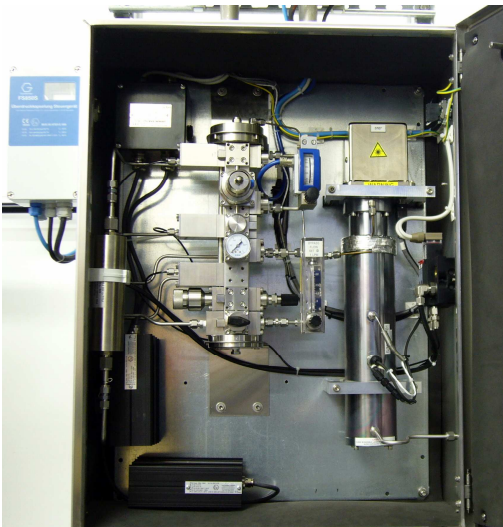
Moisture measurement by TDL
